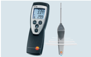
Wireless measurement with radio probes
